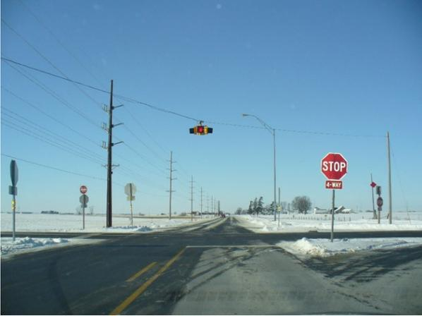
Convert two-way w/o flashing beacons to all-way stop with flashing beacons
